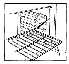
The shelves are designed with stop-locks so that when placed correctly on the shelf supports, they will stop before coming completely from the oven, and will not tilt when you are removing food from them or placing food on them.
